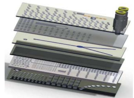
Schematic exploded view of a lab-on-Chip with microfluidic, microoptic and micro-electronic layers
